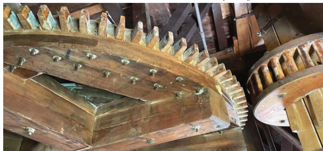
GIANT WOODEN GEARS move millstones that are located on the fifth floor of the De Zwaan windmill. The stones are still used to grind farmers' grain into flour. The windmill is made up of some 7,000 pieces, and can grind an average of 250 lbs. of flour per hour. (Photo credit: WOOD TV)
